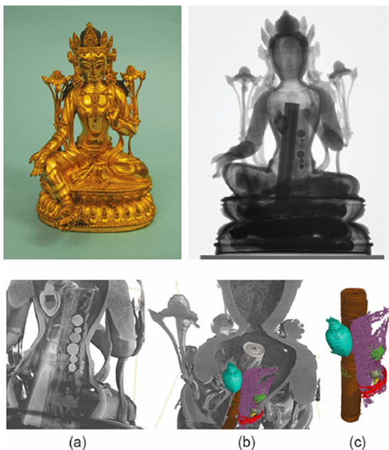
Figure 8.16: Top: Photography (a) and neutron radiography image (b) of a Buddhist bronze statue. Bottom. 3D rendering obtained by neutron tomography. (a) shows a virtual cut through the sculpture. (b) and (c) show the segmentation of three discernable objects; a small wrapped capsule (turquoise), a scroll (brown) and a pouch (violet) containing some spherical objects (green, grey, yellow) and tied up with string (red). Figure adopted from [79].
