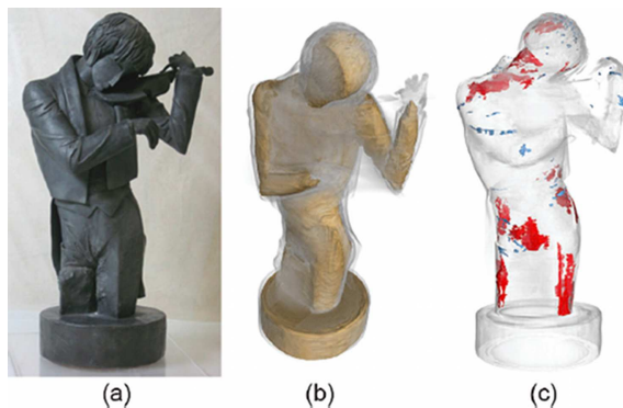
Figure 8.15: The lead and wood sculpture El violinista (1920) (a). 3D rendering of the wood core (b) and map of the areas (c) effected by corrosion (red) and needle fixations (blue) obtained by neutron tomography. Figure adopted from [79].
